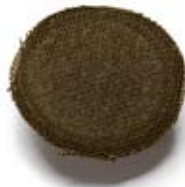
CORDURA® fabric in canvas construction 200 g/m 2 after 300,000 turns
